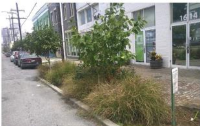
Rain Garden A rain garden is a landscaped feature designed to collect, retain, and infiltrate stormwater runoff. Rain gardens on OC Haley Blvd. are maintained by local businesses, such as Casa Borrega.
