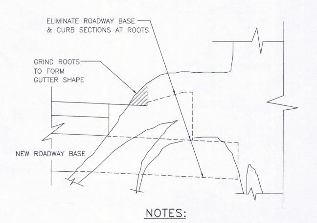
WHERE BIG ROOTS EXTEND INTO ROADWAY SECTION, ELIMINATE ROADWAY BASE AND CURB SECTIONS AT ROOTS, AND GRIND ROOTS TO FORM GUTTER SHAPE MATCHING ADJOINING CONCRETE GUTTERS AS PER DIRECTION OF THE DEPARTMENT OF PARKS & PARKWAYS
