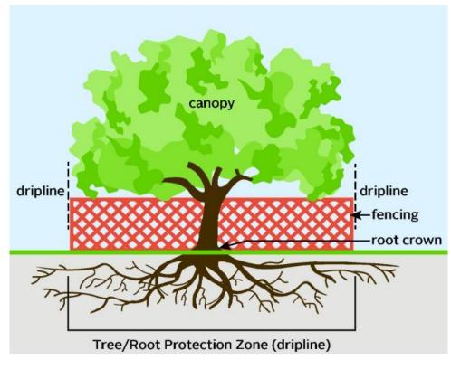
Critical Root Zone means a measurement established based on the trunk diameter at breast height (DBH). The CRZ is an equidistant circular area which has a radius calculated at one-foot to every one-inch DBH or is defined as the outer edge of the dripline, whichever distance is furthest.
