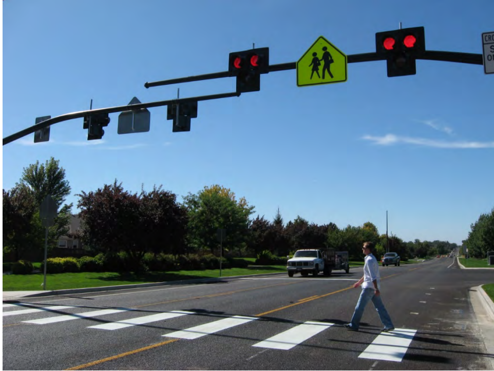
Figure 42: Example of HAWK Treatment
