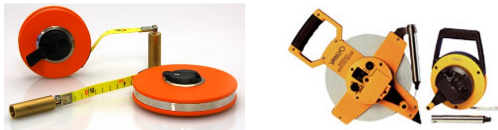
Figure 9.4 (left) low tech water level tape and plunger vs (right) water level tape with water sensor and light and sound indicators. Both accurately measure groundwater level depth from surface.
