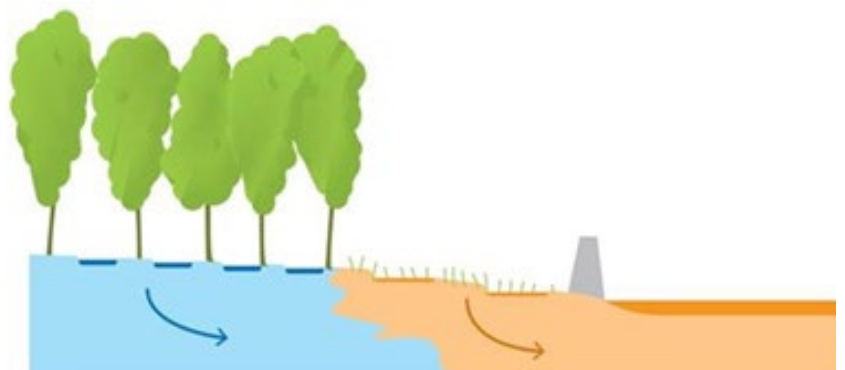
Figure 5.6 (c) Stage 3 – Civil structures and water management practices begin to transform the local ecosystem, reclaiming land by draining a section of the cypress swamp and inducing a flow reversal in the process. Now, the salty groundwater system stemming from Lake Pontchartrain now drains towards the freshwater of the cypress swamp.
