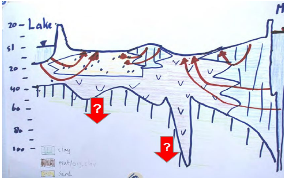
Figure 5.10 A conceptual sketch trending approximately North – South between Lake Pontchartrain and the Mississippi River in the eastern section of New Orleans. Groundwater flow lines are shown as solid red (hand drawn) arrows and lithologies such as sand, peat and clays are represented by blue, purple and yellow colors respectively.
