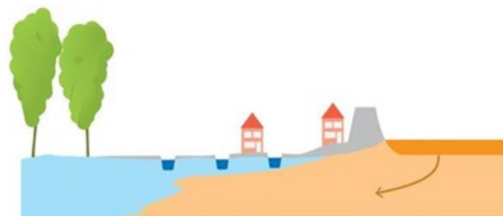
Figure 5.6 (c) Stage 3 – Civil structures and water management practices begin to transform the local ecosystem, reclaiming land by draining a section of the cypress swamp and inducing a flow reversal in the process. Now, the salty groundwater system stemming from Lake Pontchartrain now drains towards the freshwater of the cypress swamp.
