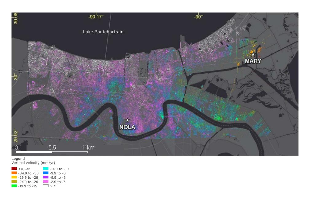
Figure 4.2. InSAR images from Jones et al. (2016). NOLA and MARY indicate Global Positioning System (GPS) Continuously Operating Reference Station (CORS) Locations.
