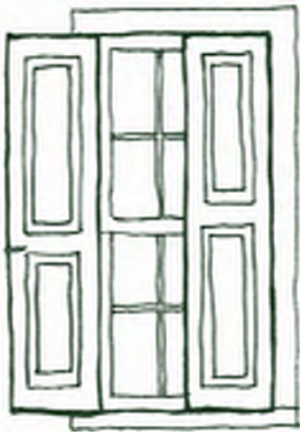
c. Paneled Shutter
