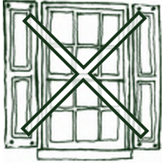
The screwed-in shutters are inoperable and all shutters should be the correct size
