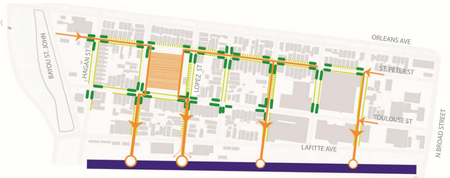
Proposed rain gardens, collection system, underground storage, and pervious sidewalks.
